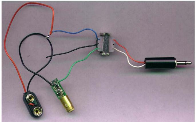
The battery clip is attached to a 4.5 volt battery pack (*not* a 9 volt battery!). Since I didn't have a pack that takes 3 cells, I used one that takes 4 AA batteries, and I replaced one of the four batteries with a straight piece of bare wire. That's it! We have a laser transmitter, in just a few minutes!
