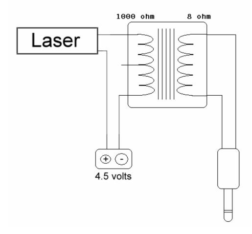
The transformer *modulates* the power going to the laser. The signal from the radio is added to and subtracted from the battery power, and the laser gets brighter and dimmer along with the volume of the music or voice in the signal. The receiver is the simplest part. You simply connect the solar cell to the microphone jack, and plug it into the amplifier or stereo phono input. It does not matter which way the wires are connected to the solar cell. Here is the schematic of the receiver:
