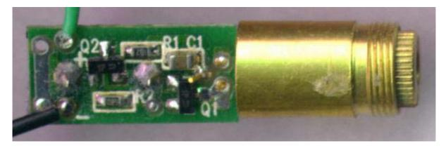
The power supply circuit came conveniently marked with a plus and a minus next to two holes in the board. We solder the black negative lead from the battery clip to the hole marked minus. We solder one of the 1000 ohm coil leads to the hole marked plus. We solder the red positive lead of the battery clip to the other lead from the 1000 ohm coil.
