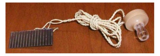
, we have tiny silicon solar cells that you can attach to a piezoelectric earphone with simple transparent tape, instead of soldering (which can be difficult to do on silicon solar cells).
