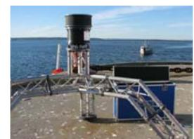
WG MIDS mounted on sea bed deployment frame.
