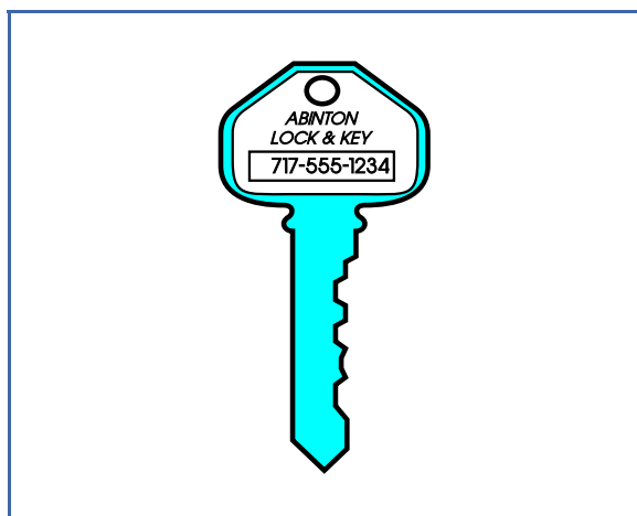
FIGURE 20—A neuter key contains no identifying information, only the name and phone number of the place where it was purchased.
