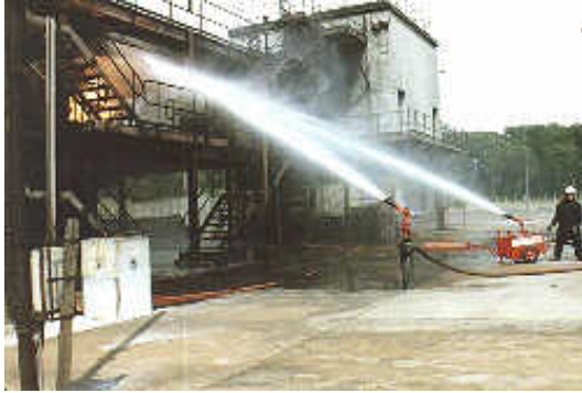
Figure 22: Strebor Portable Ground Monitors
