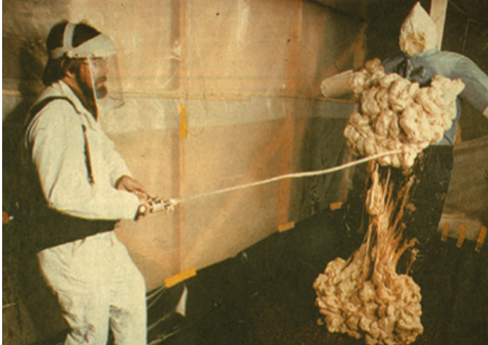
Figure 48: Demonstration of Prototype Glue Gun
