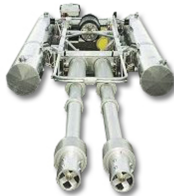
Figure 21: IFEX 18 Litre Dual Intruder Impulse Cannon
